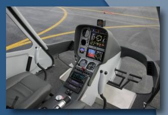
You can choose between many different avionics configurations, including moving-map GPS, dual COM, etc. At the top of the range, the new digital PFD/HSI makes the Cabri a perfect glass cockpit IFR trainer.
