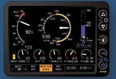
The heart of the avionics is the EPM, a dedicated multi-function display monitoring 36 parameters and providing advanced functions such as:
