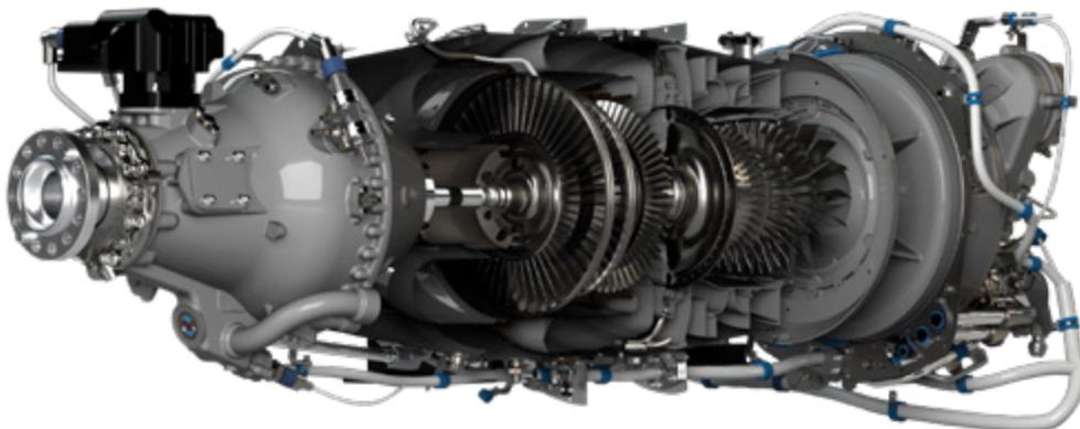
The Pratt & Whitney Canada PT6E-67XP engine combines legendary PT6 performance with the segment's first dual-channel integrated Electronic Propeller and Engine Control System featuring autothrottle. Constant monitoring of performance data yields optimal flight conditions and an increase in Time Between Overhaul intervals.
