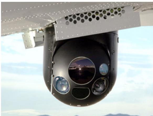
*The retractable electro-optical and infrared sensor deploys quickly in flight*
