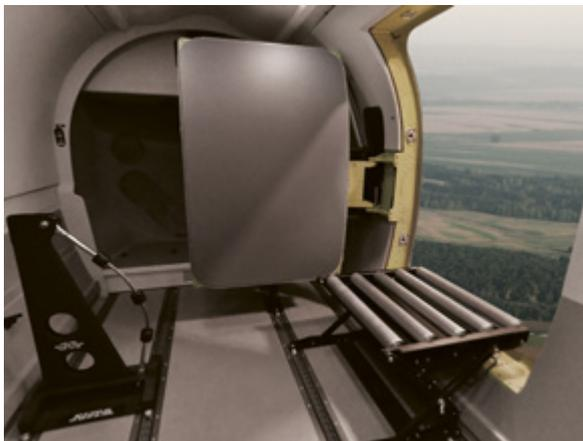
*An optional integrated utility and jump door increases the number of roles while retaining the standard cargo door functionality*
