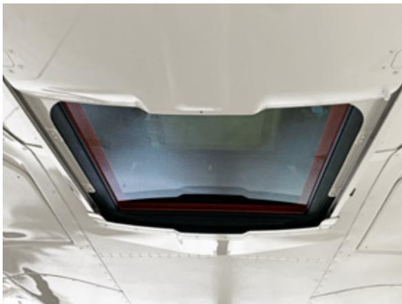
*The two hatches (21 × 21 and 21 × 9 inches/53 × 53 and 53 × 23 centimetres) can be opened in flight enabling scanning and photography*
