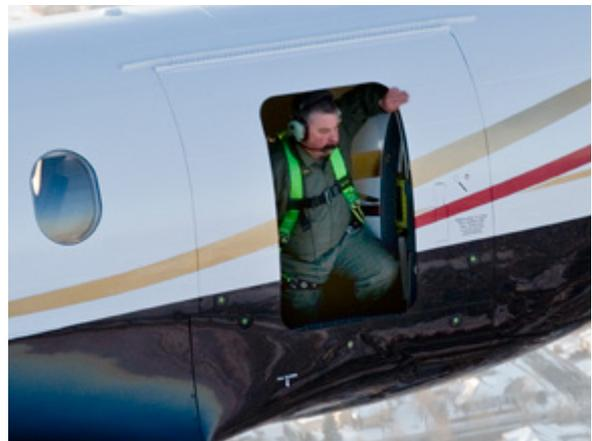
*When jump or drop operations are completed, the PC-12 NGX is re-pressurised to climb back to altitude for high-speed performance*
